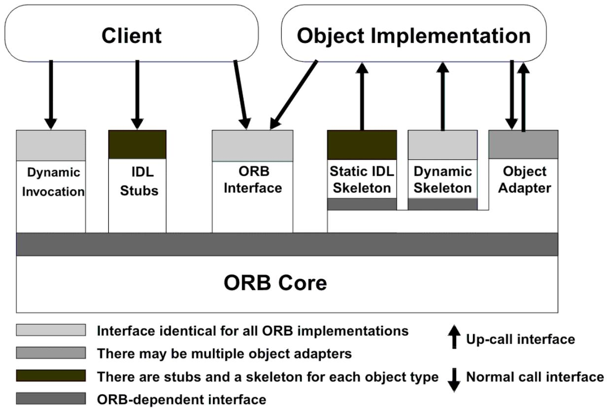
Figure 2-2 The Structure of Object Request Interfaces
